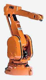
The ABB IRB 2000 is designed for fast acceleration, deceleration and top-end-speed, with a slender arm that has a reach of more than 1.5m (5 ft) and up to 3m when mounted overhead allowing for a large working envelope. When track or pedestal mounted, the IRB 2000 IRC5 can be utilized for production applications like palletizing.
