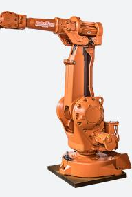
This robot offers increased production rates, reduced lead times, and faster delivery for your manufactured product. In addition, the compact design of the IRB2400 ensures ease of installation and all models offer inverted mounting capability. The IRB 2400 S4C arc welding model has a 1.5m reach and a payload of 12kg with a handling capacity up to 20kg in other models.
