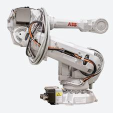
The 6-axis ABB IRB 4600-45 is proof that amazing things come in small packages. The compact design and flexible mounting options (floor, tilted, semi-shelf, or inverted) ensure space saving options and the small footprint of manufacturing cells. Your productivity and overall production capacity will increase substantially, cutting cycle times by up to 25%. The IRB 4600-45 can handle a payload of up to 45 kg and a reach of 2050 mm.
