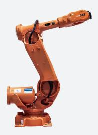
The Internal Dressing of the ABB IRB 6640ID-170 IRC5 offers higher motion control, predictable dress pack lifetime, longer dress pack lifetime, and less spare part cost. This is because the cables are routed inside the upper arm and follow the robot arm's every motion instead of swinging in irregular patterns. TrueMove and QuickMove also provide consistency as they help monitor loads and improve path precision to help increase the productivity and overall span of the robot's life.
