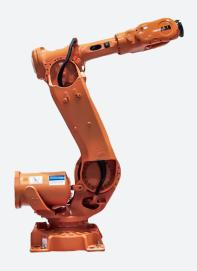
The ABB IRB 6640ID-200 is compact, with amazing inertia abilities, and perfectly designed to fit into compact places with it's 2550 mm reach and ability to fully bend over backwards. The ID models (Internal Dressing) have cable routed inside the upper arm to help reduce any external cable swinging during working hours. The ID helps to increase motion control and dress pack lifetime, reduce the footprint even more, and also decrease the spare part cost.
