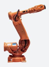
With its 2550 mm reach and 180 kg payload, the IRB 6640-180 is the perfect robot for a variety of applications such as material handling, machine tending, or spot welding. If you are in need of a robot with a big work envelope (as it can bend fully backwards), yet small footprint for a compact production line, this is the robot for you.
