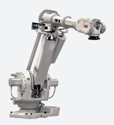
The IRB 6660 is either optimized for pre-machining or press tending. For pre-machining, the IRB6660 IRC5 has a parallel and compact mechanical design. It also has a chip protection, dedicated to increasing reliability & minimizing downtime.
