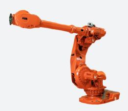
The IRB 7600/150 has a high available torque and inertia capability, rigid design, a payload capacity of 150kg, and powerful acceleration. It can be used to lift heavy pallets, handle heavy fixtures and parts, turn car bodies, lift engines, in foundries or forges, and also to load and unload machine cells.
