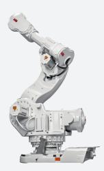
The IRB 7600/400 is a work horse robot in the 7600 family. It can handle a payload of up to 400 kg and is perfect for the next job that requires the handling of heavy and wide parts.
