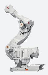
The ABB IRB 7600/500 is the robot you need to handle heavy and wide parts for a variety of applications. With a high available torque and inertia capability, rigid design, powerful acceleration, and payload capacity of up to 500 kg, no big job goes unconquered. It can be used to lift heavy pallets, handle heavy fixtures and parts, turn car bodies, lift engines, in foundries or forges, and also to load and unload machine cells.
