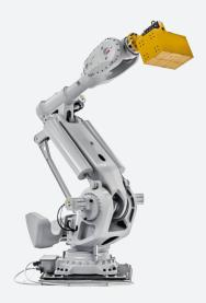
The ABB IRB 8700-550 is a highly reliable robot at an affordable price! This ABB IRB 8700  $\,$ variant has a 550 kg payload and a 4200 mm reach. With its simplified yet high quality design, this robot is easy to use and performs with ease. The ABB IRB 8700/550 IRC5 has an IP 67 and Foundry Plus 2 protection.
