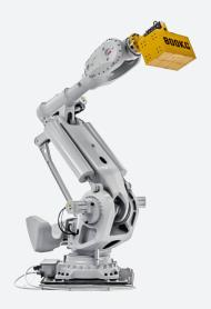
The ABB IRB 8700-800/3.5 is 25% faster than robots in its class. This ABB IRB 8700 robot is highly reliable and can handle heavy payloads up to 800 kg! The ABB IRB 8700-800/3.5 IRC5 has a 3500mm reach and a +/-0.05mm repeatability.
