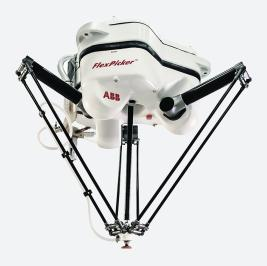
The used ABB IRB 340SA wash-down robot is built with a special paint finish, corrosion resistant materials, sealed components, and a specially designed fourth axis with slide bearings for easy cleaning. This parallel link robot is especially suited for use in packaging applications with open food.
