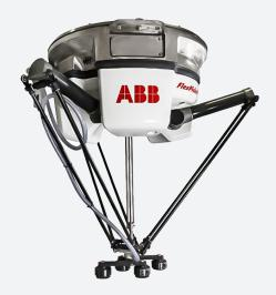
The ABB Flexpicker, the ABB IRB 360 IRC5, is a "smart' Delta robot with a compact footprint, precision accuracy, outstanding motion control, and short cycle times. The IRB 360 operates in narrow to wide spaces with tight tolerances, all at very high speeds.
