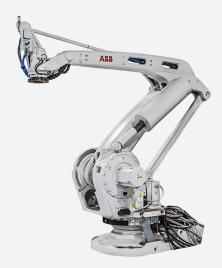
The ABB IRB 660-250 is the high throughput version that is designed to tackle palletizing jobs in shorter cycle times. Its speed, 250 kg payload, and 3150 mmm reach allow it to serve up to four in-feed conveyors, two pallet stacks, one slip-sheet stack, and four palletizing out-feeding lines. The IRB 660-250 truly has the versatility, reach, and handling capacity to become the ideal solution for all palletizing applications including palletizing bags, boxes, crates, bottles, and more.
