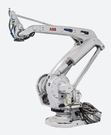
The ABB IRB 660 is engineered to meet the automation requirements for robot-based packaging lines. It is devised increased productivity solutions. The ABB IRB 660 is highly precise and efficient. The ABB IRB 660 has a state-of-the-art 4 axes design. Its optimized motor power and motion performance ensures significantly shorter cycle times.
