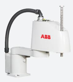
The ABB IRB 910SC - 3/0.55 robot is the ideal solution for customers that are seeking faster cycle times, amazing precision, and excellent reliability. The ABB IRB 910SC - 3/0.55 provides a 550 mm reach that operates within a small footprint, saving production floor space. A few other benefits of the IRB 910SC-3/0.55 include the fact that it is modular, table top mountable, and IP54 rated.
