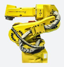
The FANUC Arc Mate 100iB/6S features a 6kg payload, 951mm reach, and comes equipped with the RJ3iB controller and teach pendant.
