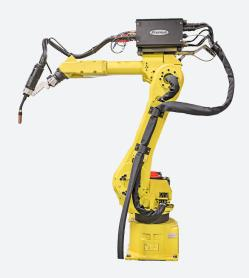
The FANUC ARC Mate 100iB is a six-axis, modular construction, electric servo-driven welding robot that was designed with high speed in mind. Compact and flexible, the Arc Mate 100iB robot is capable of high speed welding and cutting, yet precise enough to handle pick and place applications. The FANUC ARCMate 100iB has a relatively lightweight payload ability at 6kg, which makes it perfect for welding applications.
