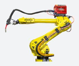
The extended reach FANUC ARC Mate 120iB/10L performs arc welding and cutting applications with ease. The 120iB/10L uses its six-axes, overhead rail-mount, horizontal reach of 1,885 millimeters and, +/- 0.1 millimeter repeatability to ensure that parts large and small receive extremely accurate welds and cuts. The FANUC ARC Mate 120iB/10L R-J3iB arc welding robot has a maximum payload capacity of 10 kilograms.
