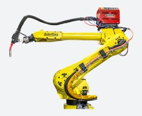
The FANUC ARC Mate 120iBe welding robot has six axes, a remarkable reach/stroke ratio and elevated axis speeds. The controller has been integrated into the base of the robot to simplify installation and conserve production floor space. All FANUC 120iBe R-J3iC basic arc welding robotic software features are supported to provide superior performance for simple and complex arc welding applications.
