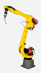
The FANUC ARC Mate 120iC/12L is a long reach robot, specifically designed for arc welding. The ARC Mate 120iC/12L has a long arm, allowing a reach up to 2009 mm. It is the highest motion performance robot for its class, yet maintains a slim and compact design to help reach those tight spaces. Featuring a hollow wrist for the torch cable integration, unique wrist design, and 12kg payload, this robot produces at the utmost speed while providing easy management.
