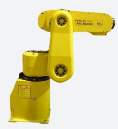
The FANUC ARC Mate 50iB/3L arc-welding robot features a long reach for maximum flexibility. The ARC Mate 50iB/3L R-J3iB welding robot has an 856 mm horizontal reach allowing for a wide work envelope. With a +/- 0.04 mm repeatability and a 3 kg maximum payload capacity, a light-weight arc welding torch will weld parts with extreme accuracy and precision.
