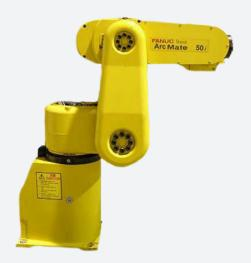
The FANUC ARC Mate 50iB is a six-axis robot engineered to offer versatility in a simple package. A tabletop welder with a low 47kg mass, the ARC Mate 50iB RJ-3iB is designed to perform high-speed arc welding applications.
