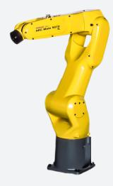
The FANUC ARC Mate 50iD/7L is a high speed arc welding robot that is equipped with added reach. The FANUC ARC Mate 50iD 7L has a long arm and +/-0.03mm repeatability. With 6 axes, this Arc Mate 50iD/7L robot can carry up to 7kg while creating precise arc welds.
