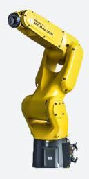
The FANUC ARC Mate 50iD robot is a compact arc welding robot that is equipped to operate in dusty or wet environments. The wrist of the ARC Mate 50iD has an IP67 rating, which means it is totally protected against dust, while also being protected against the effects of immersion in water between 15cm and 1m. The 50iD also has an optional IP69K rating for the body, J3 axis, and wrist, which makes the robot arm able to withstand high pressure steam cleaning as well.
