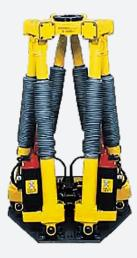
Suitable for light to medium material handing processes, the FANUC F-200iB is a six degrees of freedom servo driven parallel link robot. The FANUC F-200iB R-J3iB is engineered in a compact package for applications requiring extreme rigidity and exceptional repeatability. The FANUC F-200iB R-J3iB is capable of a wide variety of material handling tasks.
