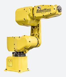
The FANUC LR Mate 200iB/5C is a six-axis, electric servo-driven cleanroom assembly and industrial robot. The tabletop size provides the Mate 200iB/5C R-J3iB with dexterity and high speed. The LR Mate 200iB/5C is capable of a wide variety of tasks in a broad range of industrial and commercial applications including machine tending and part handling.
