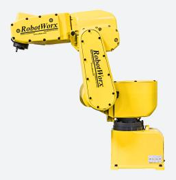
The versatile FANUC LR Mate 200iB is a compact, modular construction, table-top robot that can be used for a variety of applications. The 200iB robot is electric servo-driven and has a six-axis arm with many different mounting capabilities. The 200-iB also has the ability to flip over backwards for a larger work envelope and to provide maximum flexibility.
