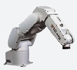
FANUC's LR Mate 200iC/5F robot provides an entry for industrial automation in primary and secondary food handling work environments. The LR Mate 200iC/5F R-30iA has an option to be clean-room friendly and uses only food-grade grease. It is also sealed at every axis joint to give it an IP67 rating.
