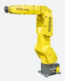
FANUC LR Mate 200iC/5L robots are used for a wide variety of applications such as machine tending, material handling, assembly, dispensing, and material removal. It is a tabletop robot with a long reach of 892 mm and is designed with a slim wrist and a small footprint, aiding it in reaching confined places. It is rated best-in-class for performance in a light, efficient, accurate, and nimble (LEAN) package.
