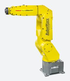
Faster and more compact than its predecessors, the FANUC LR Mate 200iC robot arm's high-positioning accuracy and tabletop size make it ideal for a variety of automation applications, including material handling, machine tending and assembly. The size of a human arm, the mini LR Mate 200iC moves with 152 percent more speed and 50 percent more accuracy than the earlier models.
