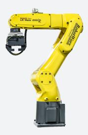
The FANUC LR Mate 200iD/7L is the long reach version in the LR Mate 200iD series displaying a reach of 911 mm. This is a high motion performance robot with a wide work envelope and is great for a wide variety of applications, such as material handling, polishing, pick and place, or assembly. This compact, multi-purpose robot is also very fast at handling small payloads up to 7 kg. The 200iD/7L has an enhanced wrist load capacity for great efficiency and ability to handle multiple workpieces.
