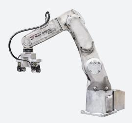
The FANUC LR Mate 200iD/7WP has an IP67 rating standard, with an IP69k option as well, which means that the robot is dust-proof, but it can also handle immersion in water up to 1 m, and it can handle high pressure cleaning from steam jets. This type of cleaning is important for robots like the LR Mate 200iD/7WP, especially when being used in food and pharmaceutical environments, as mentioned above.
