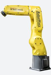
The FANUC LRMate 200iD is the latest, compact, mini robot that has the approximate reach and size of a human arm. This helps to minimize interference with peripheral devices and allows operation in narrow spaces. It is known as the lightest mechanical unit in its class and has multiple mounting options which helps with installation flexibility.
