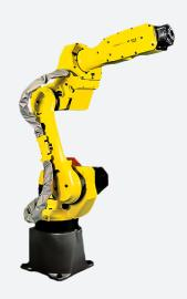
The FANUC M-10iA/10MS is a high speed, short arm robot ideal for a variety of applications, including material handling, bonding/sealing, packaging, cutting, and more! The M-10iA/10MS is a highly reliable robot with an RV reducer and gear and harmonic drive trains to help enhance the rigidity and performance. Furthermore, there is minimal maintenance with the sealed bearings and brushless AC motors.
