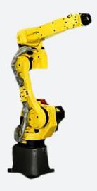
Great for a variety of applications, the FANUC M-10iA/10S might be a short arm, but it has a great might! The FANUC M10iA/10S has a 10 kg payload and +/- 0.05 repeatability, with the highest wrist moments and inertia in its class, making a it a high performance industrial robot.
