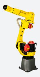
The FANUC M-10iA/12S has the best payload and inertia in its class! It is the short arm version of the M-10iA/12 that provides a 1098 mm reach and a slim and hollow arm and wrist. It can be mounted at a variety of angles on the floor or wall, or ceiling mounted, ultimately making this robot the perfect for accessing difficult angles and narrow spaces.
