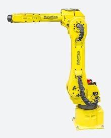
Designed to perform many material handling applications, the FANUC M-16iB/20 features a payload capacity of 20 kilograms. It has servo driven motors, a simple construction, and reliable motion control that further improved productivity and performance.
