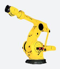
The M-2000iA/1700L from FANUC is one of the strongest long reach robots in the world. It is typically used in machine tending, material handling, machine loading, and material removal applications.
