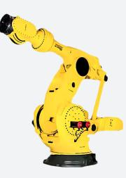
This robot is the strongest lifter in the FANUC family, with a payload capacity to lift 2.3 metric tons of product -- meaning it could easily lift an entire car and move it to a different area on the factory floor. The steady motion of the robot, with its low vibrations, means that the jerking movements of cranes or other lifters are things of the past. The low noise level and moderate power consumption (8 kW) are also benefits that the M-2000iA/2300 bring to the table.
