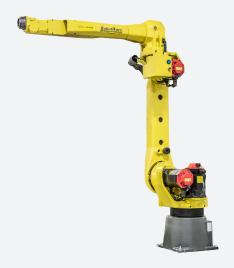
The FANUC M-20iA/10L is an industry leader in reliability. The hollow upper arm and wrist of the M-20iA series helps to answer these problems as utilities are permitted to be contained within the arm, helping to eliminate snagging, tearing, or rubbing. There is also a shelf on the back of the upper arm that enables peripheral equipment to be easily mounted. There is also a built-in vision cable from J1 to J3 allowing an easy transition for the addition of a vision application.
