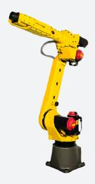
The FANUC M-20iA/35M is ideal for a variety of applications ranging from material handling to assembly. With the ability to handle 35 kg, this M20iA robot can offer more strength. The M20iA/35M has a 1,813 mm reach and 0.08 mm repeatability. The M-20iA/35M is able to decrease down-time caused by dress out as it has a hollow upper arm and wrist that neatly contains the cables. This eliminates any snagging, tearing, or rubbing and makes it perfect for offline programming.
