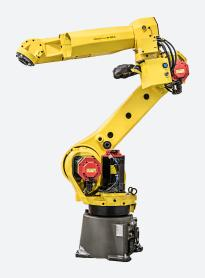
The M-20iA has a hollow upper arm and wrist and a unique design that enables utilities to be neatly contained within the arm, helping to avoid snagging, tearing, or rubbing. The M-20iA has built-in vision with an integrated vision cable from the J1 base to J3 interface panel, making the addition of vision to the robot application much easier.
