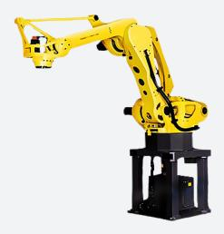
The FANUC M410iC/500 comes equipped with a R-30iB controller and an intelligent iPendant Touch and has a protection rating of IP54, which means it has complete protection against contact, some protection against dust, and splashing water, which allows it to work in a variety of different places on a factory floor. Cables and hoses are routed through the robot's wrist, which keeps cables from swinging and snagging on other existing structures or robots.
