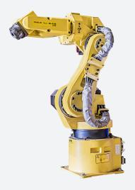
The M-6iB/2HS is a high speed variant, with greater throughput, of the M-6iB series, yet it maintains the same compact size, slim wrist, and small footprint in the series. Because the FANUC M6iB/2HS has a lighter payload, its speeds are much faster, as it can be used for rapid pick and place operations.
