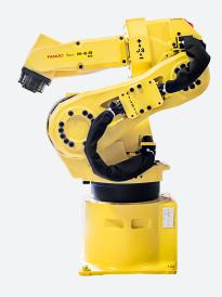
The FANUC M-6iB/6S is a short arm robot arm designed for compact, confined spaces. The M6iB/6S R-J3iB robot arm performs material handling tasks where parts sizes and work envelopes are less of an issue. A +/- 0.08 millimeter repeatability and a 6 kilogram maximum payload capacity allow the M 6iB/6S to perform precise, lightweight material handling.
