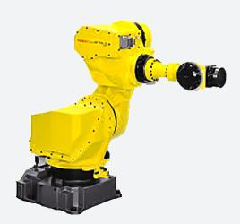
The FANUC M-710iB/45 features a 45 kg payload and 1706mm reach. This FANUC M710iB/45 comes equipped with the intelligent R-J3iB controller. This robot is fast and efficient and can perform a wide variety of applications ranging from material handling to dispensing, Furthermore, the M-710iB/45 can be mounted on the floor, ceiling, or at an angle. Its compact size allows for a smaller footprint and its AC servo motors with high power to weight proportions allow for very fast speeds.
