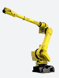
The FANUC M-710iC/20M is a compact robot capable of a variety of applications, including arc welding and material handling. The FANUC M710iC/20M has a slim wrist, rigid arm, and a small footprint. It has a payload of 20 kg, reach of 2,582 mm, and can perform at very high speeds.
