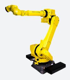
The FANUC M-710iC/50E features an offset wrist design that makes it an ideal fit for grinding and polishing applications, while the payload and rigid arm make it a great robot for deburring, machine tending, and waterjet cutting applications as well.
